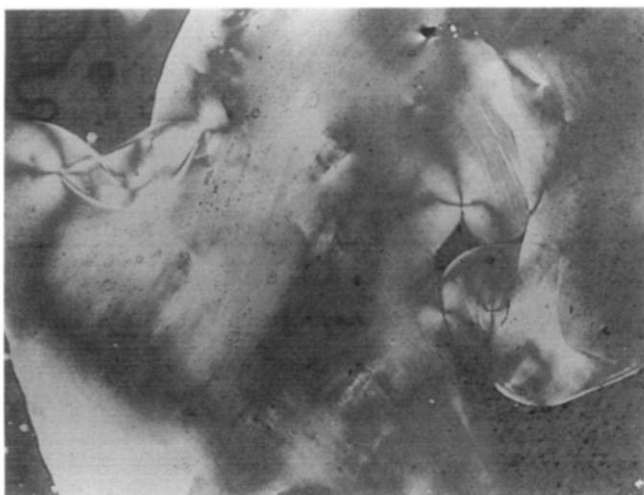
Figure 8 Photomicrograph of C_8 polymer at 138^\circ\text{C} (under light pressure) in the heating cycle ( \times 57 )
